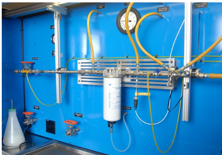
Test filter installation configured for ISO 16332
